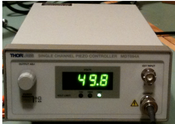
Figure F.6: High voltage (HV) amplifier (THORLABS model MDT694A). The display shows the output voltage. A voltage applied to the “EXT INPUT” on the front is amplified and that voltage is added to that set by the manual “OUTPUT ADJ” knob. The input multiplier changes depending on the voltage limit indicated by the green LED.
